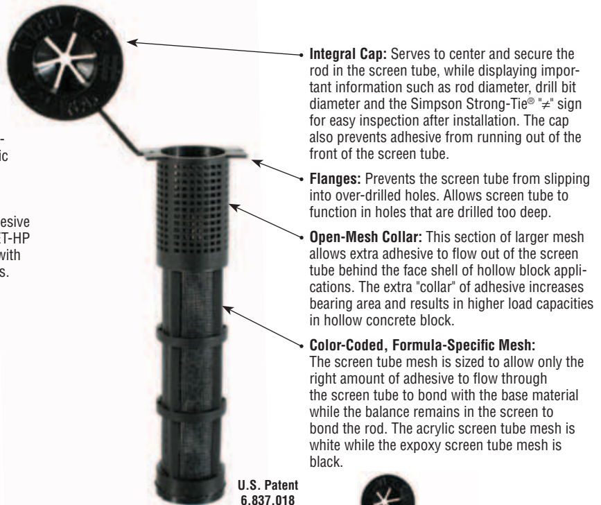
Epoxy Screen Tube (mesh is black)
